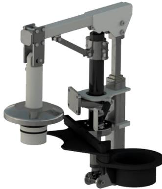
The telescoping night cap extractor arm provides a simple and effective way to add or remove the night cap from the Lee Posi Lock. A docking station is attached to hold the night cap when not in use. With the telescoping design, as long as the lubricator remains above the funnel, it will not swing into the Lee Lock.
