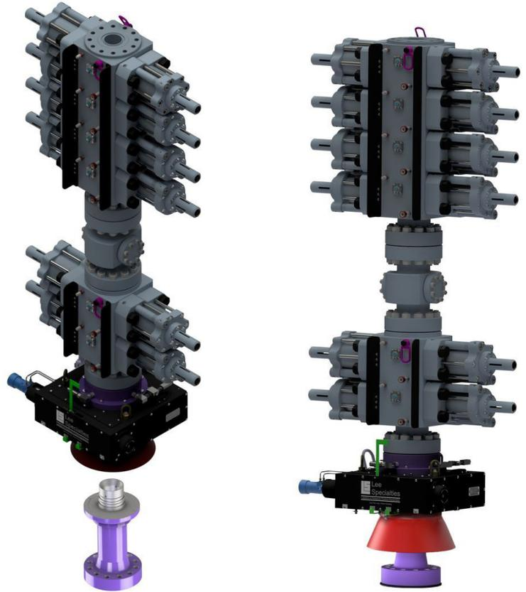
The Coil Posi Lock stinger allows for insertion into the funnel of the lock and further into the lock where it is then clamped. It can be fitted to the wellhead or at any point in the pressure control stack which would benefit from a remote quick connection. The stinger is available in most common quick unions and API flanged connections.
