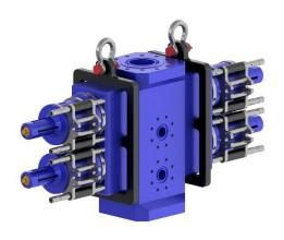
Lee Specialties manufactures hydraulically actuated coiled tubing BOP's which require hydraulic pressure to open and close the rams. This feature allows for safer and more efficient operation from a location removed from the pressure stack and wellhead. The hydraulic supply system can be a two-way hydraulic hand pump or an accumulator system. Quick connect unions available upon request.
